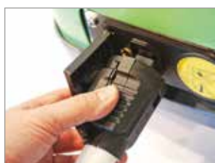
STEAM HOSE HOOK EQUIPPED WITH SAFETY PANEL
