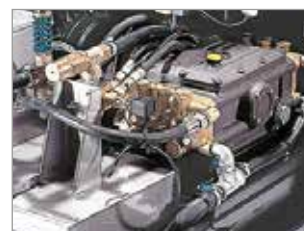
PLUNGER PUMP WITH SIX CERAMIC PISTONS AND TWO BRASS HEADS
