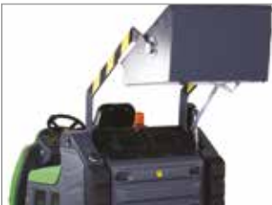
HOPPER HYDRAULIC DISCHARGE SYSTEM
