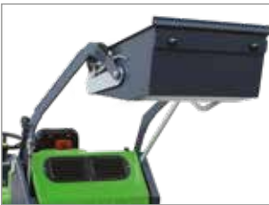
HOPPER HYDRAULIC DISCHARGE SYSTEM
