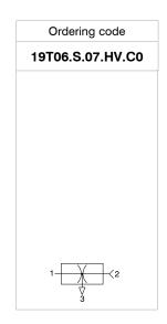
Single stage generators, with operation based on the Venturi principle; their main feature is the presence of feed pressure and connection for the vacuum on the same axis. This makes it possible to connect the suction cups directly to the generator or through the suction cup holder, so therefore still on the same axis with obvious advantages in terms of system layout and simplicity.
