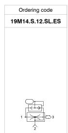
High-performance compact generator for high frequency applications; the presence of the integrated ejector ensures release capacity in the shortest possible time. The fact of it being extremely lightweight allows its application directly onto the robot gripping arms and/or mobile applications. Available with two flow rates in the same overall dimensions.
