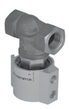
The valves are composed of a bronze body, 2 ways, with pneumatic control, with a compact single or double acting cylinder with connections which can be turned 360°. Versions are available that have the gaskets in contact with the fluid, and are made of NBR, FPM or PTFE.
