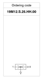
Single stage high suction power generators operating using a single large Venturi nozzle; particularly silent thanks to a free-low silencer which is mounted separately. Suitable for use in dusty environments and in applications where a large suction capacity and a high degree of vacuum are required (92 -kPa).
