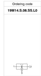
Single stage generators, with operation based on the Venturi principle; their main feature is the presence of feed pressure and connection for the vacuum on the same axis. This makes it possible to connect the suction cups directly to the generator or through the suction cup holder, so therefore still on the same axis with obvious advantages in terms of system layout and simplicity. The outlet connection has a female thread G 1/8".
