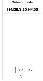
Single stage high suction power generators operating using a single large Venturi nozzle; particularly silent thanks to a free-low silencer which is mounted separately. Suitable for use in dusty environments and in applications where a large suction capacity and an average degree of vacuum are required (57 -kPa).
