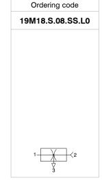
Single stage generators, with operation based on the Venturi principle; their main feature is the presence of feed pressure and connection for the vacuum on the same axis. This makes it possible to connect the suction cups directly to the generator or through the suction cup holder, so therefore still on the same axis with obvious advantages in terms of system layout and simplicity. The outlet connection has a female thread G 1/8".
