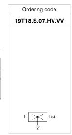
Single stage generators, robust and reliable, with compact dimensions and suitable for applications which need the required degree of vacuum to be reached quickly with limited air flows. Operating on the Venturi principle they have the vacuum connection orthogonal to the axis of supply and outlet. They can be connected directly to the suction cups and/or suction cup holder and applied in any position.
