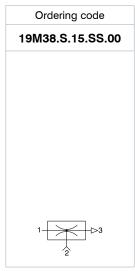
Single stage generators, robust and reliable, with compact dimensions and suitable for applications which need the required degree of vacuum to be reached quickly with limited air flows. Operating on the Venturi principle they have the vacuum connection orthogonal to the axis of supply and outlet. They can be connected directly to the suction cups and/or suction cup holder and applied in any position.
