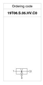
Single stage generators, with operation based on the Venturi principle; their main feature is the presence of feed pressure and connection for the vacuum on the same axis. This makes it possible to connect the suction cups directly to the generator or through the suction cup holder, so therefore still on the same axis with advantages in terms of system layout and simplicity.
