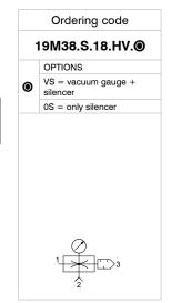
Single stage generator with high suction capacity due to a pair of nozzles mounted in parallel; they are particularly quiet thanks to a free-flow type silencer, standard-fitted with a vacuum gauge, and allows direct connection with a vacuum switch or alternatively a solenoid valve for quick detachment via direct blowing into the vacuum connection. Suitable for decentralised connection of one or more suction cups.
