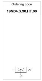
Single stage high suction power generators operating using a single large Venturi nozzle; particularly silent thanks to a free-low silencer which is mounted separately. Suitable for use in dusty environments and in applications where a large suction capacity and an average degree of vacuum are required (57 -kPa).
