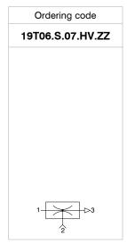
Single stage generators, robust and reliable, with compact dimensions and suitable for applications that need the required degree of vacuum to be reached quickly with limited air flows. Operating on the Venturi principle they have the vacuum connection orthogonal to the axis of supply and outlet. They can be connected directly to the suction cups and/or suction cup holder and can be applied in any position.
