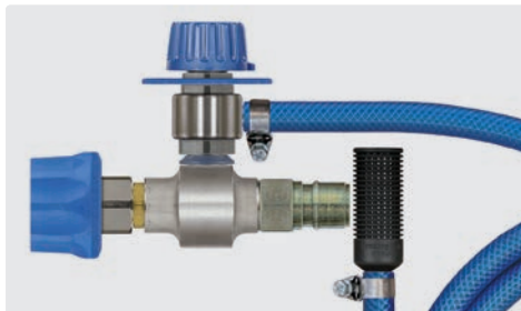
Coupling ST-45-250 nickel-plated brass : plug ST-45-250 zinc-plated steel. Injector with metering valve ST-161, suction hose 2,000 mm and suction filter ST-31. Max. 250 bar / 90 °C
