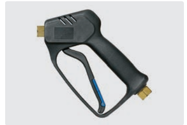
Professional gun. Weep version. Max. 210 bar / 25 l/min / 150 °C
