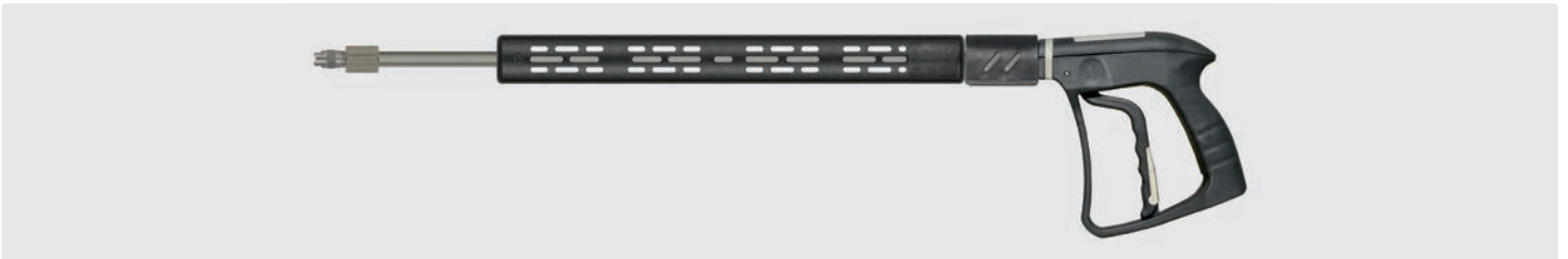
Professional steam gun with lance stainless steel, vented handle ST-9 380 mm and steam low pressure nozzle made out of stainless steel. Max. 20 bar / 200 °C
