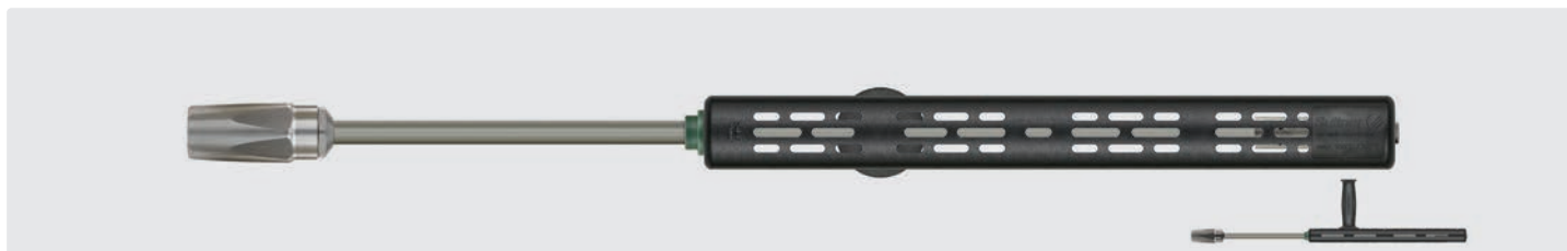
1/4" M. Foam lance stainless steel with air injector, vented handle ST-9 380 mm, grip and stainless steel socket with nozzle. A foam injector is required. Max. 250 bar / 80 °C
