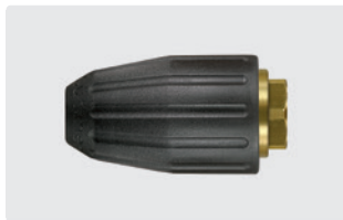
1/4" F. Spray angle 20°. 200 - 350 bar. Max. 100 °C
