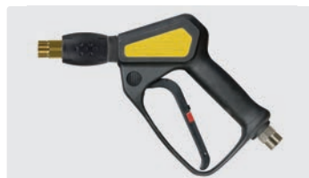
Professional gun with Variopress. Variopress regulates the water quantity and serves for the adjustment of pressure. Max. 310 bar / 45 l/min / 150 °C
