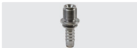
Crimp nipple. DN 4. M7x0,5 M. Stainless steel. Max. 500 bar
