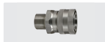
Coupling : M. Stainless steel. 60° cone. Max. 250 bar / 150 °C
