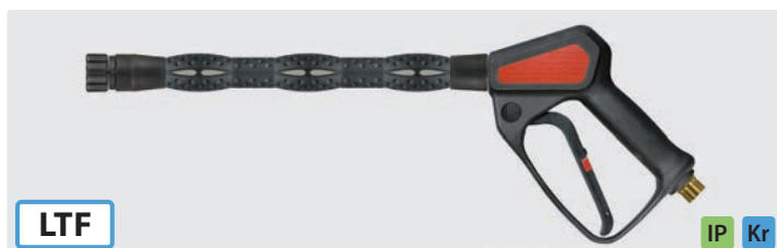
Professional gun with patented LTF technology. Gun with extension ST-9.1 350 mm and M22 F. Max. 310 bar / 45 l/min / 150 °C
