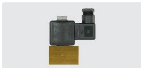
1/4" F. NW 1.5 mm. Solenoid valve with connector. Pressure range 0 - 130 bar. Max. 90 °C
