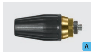
1/8" M. Spray angle 20°. 100 - 250 bar. Max. 100 °C
