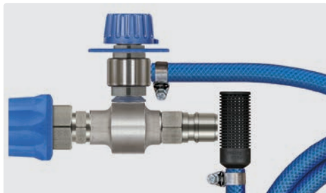
Coupling ST-45-250 stainless steel : plug ST-45-250 stainless steel. Injector with metering valve ST-161, suction hose 2,000 mm and suction filter ST-31. Max. 250 bar / 90 °C
