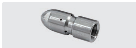
M7x0,5 F. ⚙ rear jets for maximum thrust. Additional 3 side jets (90°) for powerful cleaning impact and optimal wall coverage. Outside \varnothing 9.8 mm. Stainless steel. Max. 500 bar
