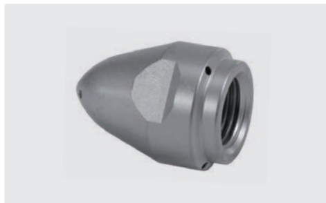
Outside \varnothing 22 mm. Hardened stainless steel. Max. 500 bar / 35 l/min.
