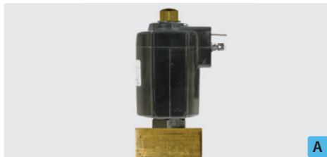
1/4" F. NW 1.2 mm. Solenoid valve without connector. Pressure range 0 - 180 bar. Max. 90 °C
