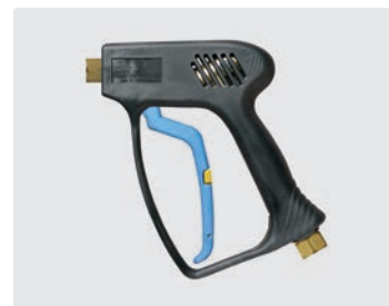
Professional gun. Weep version. Max. 275 bar / 45 l/min / 150 °C
