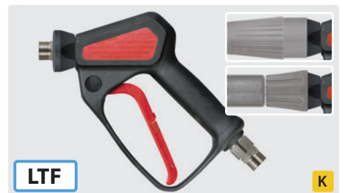
Professional ultra high pressure gun with patented LTF. Gun with insulated outlet suitable for lances with swivel screw coupling. Max. 500 bar / 30 l/min / 150 °C
