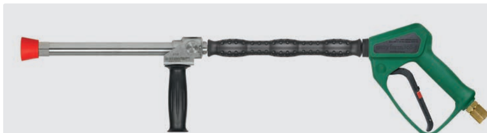
1/2" F. Stainless steel. Longcast lance 350 mm with insulation ST-29 Cool & Compact 330 mm, gun easyfarm365+, grip aside and nozzle protector made out of plastic without nozzle. Max. 250 bar / 60 l/min / 100 °C
