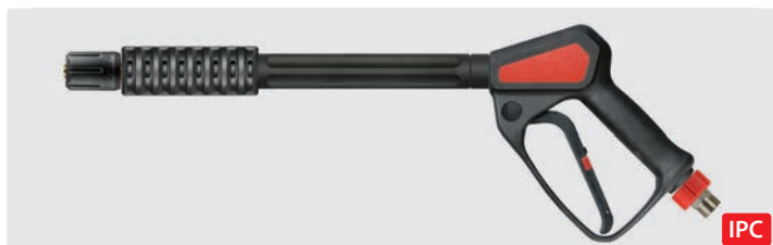
Professional gun with extension 340 mm and M22 F. Max. 310 bar / 45 l/min / 150 °C
