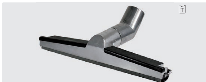
All-purpose nozzle IRD 500. Vacuum tool with brush strips, rubber lips and height adjustable rollers. Aluminium. For all carpets and hard covers
