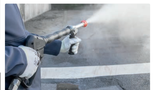
1/4" M. Stainless steel. Longcast lance 350 mm with insulation ST-29 Cool & Compact 330 mm, grip aside and nozzle protector made out of plastic without nozzle. Max. 280 bar / 130 l/min / 100 °C
