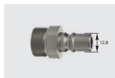
Plug : M. Stainless steel. Max. 350 bar / 100 °C
