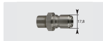
Plug : M. Stainless steel. 60 °Cone. Max. 250 bar / 150 °C
