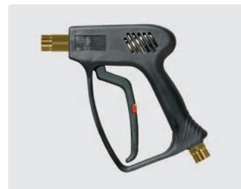
Professional gun. Max. 275 bar / 45 l/min / 150 °C
