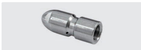
M7x0,5 F. ⚙ rear jets for maximum thrust and powerful cleaning impact. Outside \varnothing 9.8 mm. Stainless steel. Max. 500 bar
