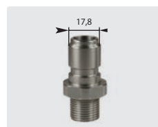
Plug : M. Stainless steel. 60° cone. Max. 250 bar / 150 °C
