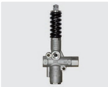
Stainless steel. \odot = inlet 1/2" F. \ominus = outlet 1/2" F. \square = bypass 1/2" F. Max. 600 bar / 90 °C
