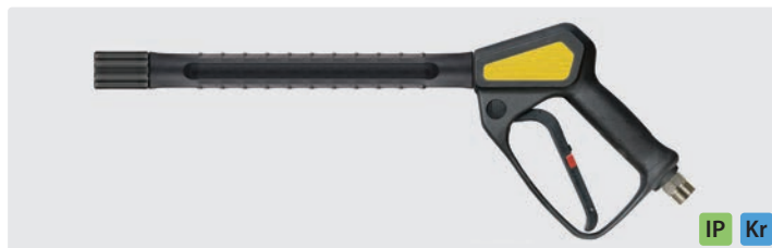
Professional gun with extension ST-9.9 370 mm and M22 F. Max. 310 bar / 45 l/min / 150 °C
