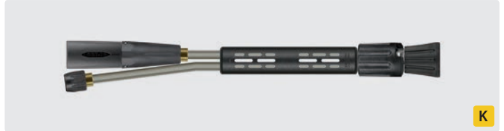
Twin foam lance with vented handle ST-9 205 mm, change-over valve ST-58, ergonomic swivel screw coupling, nozzle protector without tip and foam head ST-75.1 without nozzle. A foam injector is required.
