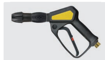
Professional gun with Variopress and coupling KW. Variopress regulates the water quantity and serves for the adjustment of pressure. Max. 310 bar / 45 l/min / 150 °C
