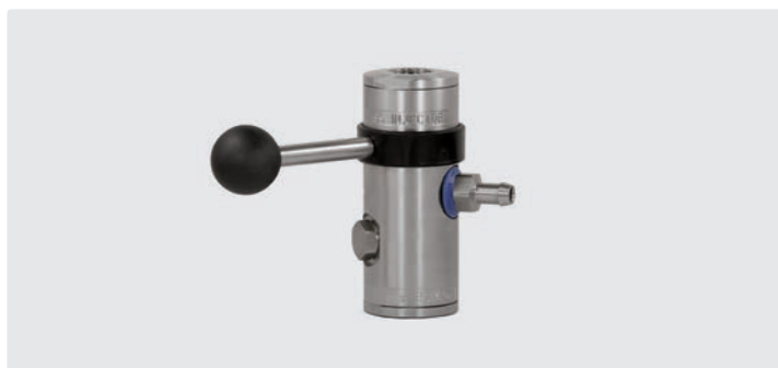
1/2" F : 1/2" F : hose tail 9 mm. The chemical dosing is adjusted by 10 exchangeable nozzle inserts (0.5 - 2.0 mm).
