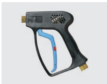
Professional gun. Freeze stop version. Max. 275 bar / 45 l/min / 150 °C
