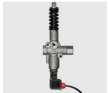
Stainless steel. \odot = inlet 1/2" F. \ominus = outlet 1/2" F. \square = bypass 1/2" F. Regulation valve with switch (IP55) and cable 950 mm. Max. 600 bar / 90 °C
